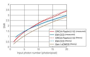
The ORCA-Flash4.0 V2 SNR exceeds that of EM-CCDs at about 6 photons/pixel. The solid lines show measured data at 533 nm. This measurement aligns well with predicted values (dotted line) for EM-CCD and ORCA-Flash4.0 V2. For
