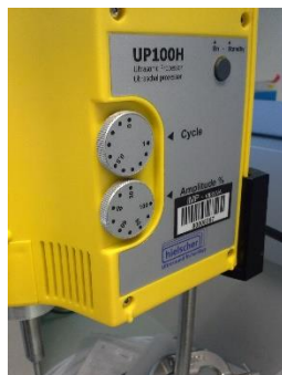
Picture 3: Sonicator probe with right settings
