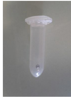
Picture 2: Tungsten bead in 2mL Eppendorf tube
