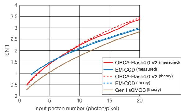
The ORCA-Flash4.0 V2 SNR exceeds that of EM-CCDs at about 6 photons/pixel. The solid lines show measured data at 533 nm. This measurement aligns well with predicted values (dotted line) for EM-CCD and ORCA-Flash4.0 V2. For comparison, the theoretical line for the Gen I type sensor is shown. Due to low QE and higher read noise, the Gen I camera does not compete with EM-CCD or Gen II ORCA-Flash4.0 V2 at these low light levels.
