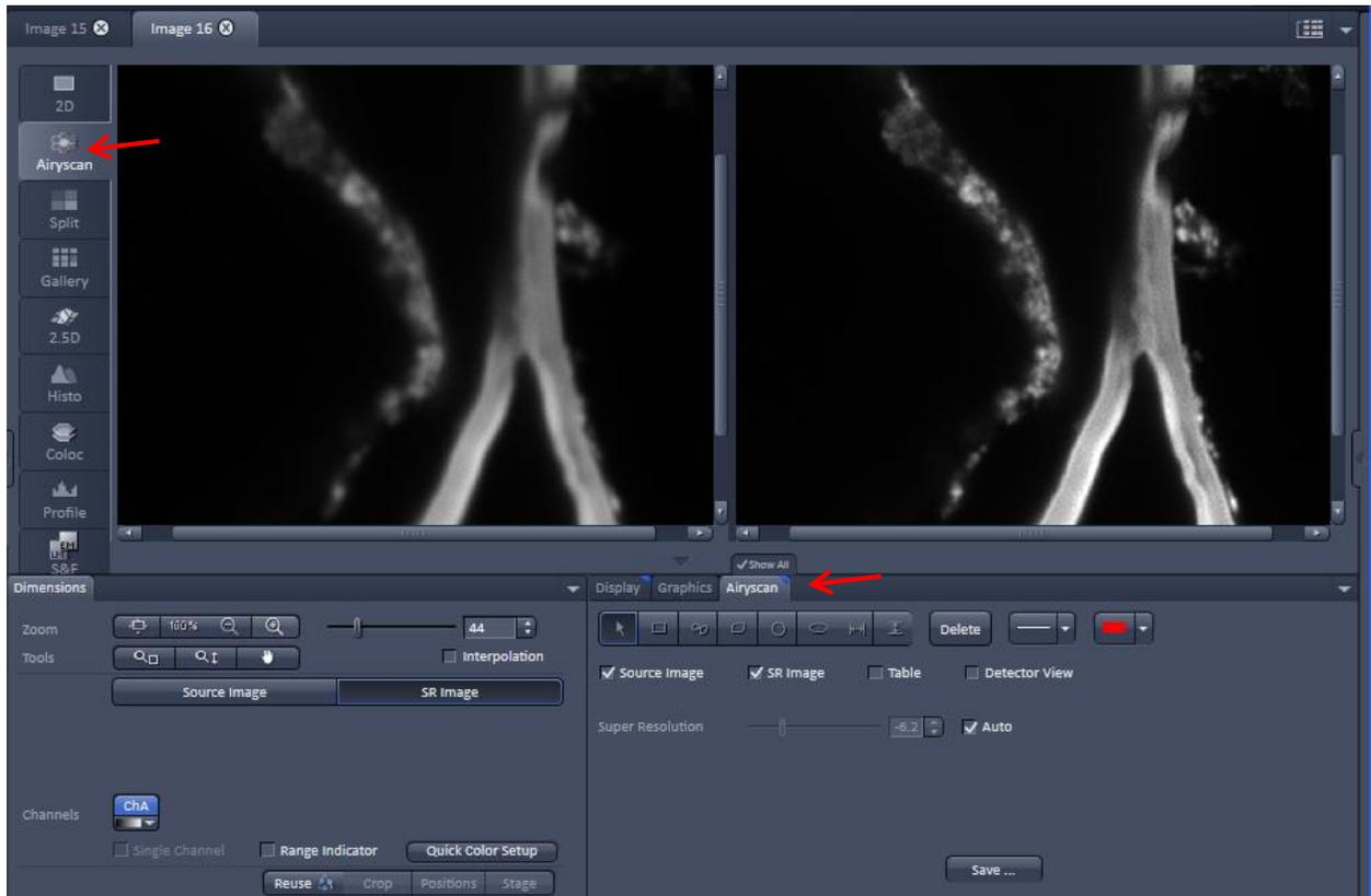
2. Activate Source image and SR image. The source image shows the same as 2D, an average of all detector elements and the SR image shows the SR image of the current z-plane.
