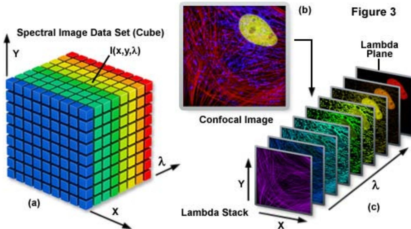
Fig. 2. Description of a spectral image data set. Each point in the cube represents a single number and the spectral image is described as  $I(x,y,\lambda)$ . It can be viewed either as an image  $I(x,y)$  at each wavelength  $\lambda$ , or as a spectrum  $I(\lambda)$  at every pixel  $(x,y)$ .
