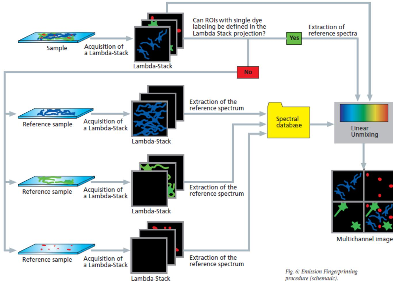
Fig. 6: Emission Fingerprinting procedure (schematic).
