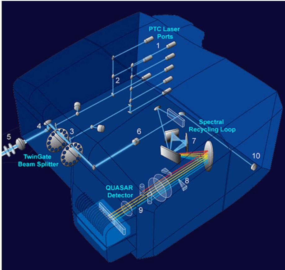
34 Channel QUASAR detection unit used in *Lambda Mode*
